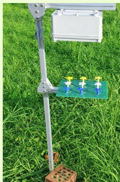
Figure 1: Camera trap and compute module integrated into the RoofPoll monitoring system (schematic view) © Dr. Hanna Honchar
